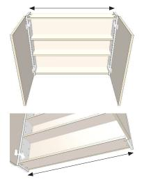
Bottom/Deck is set up from left and right end panels
