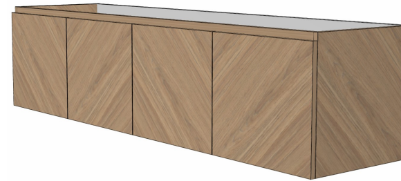
Render above indicates grain direction on fronts and side panels
